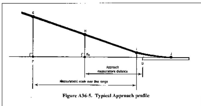
The airplane reference point for approach measurements is the instrument landing system (ILS) antenna. If no ILS antenna is installed an alternative reference point must be approved by the FAA.
