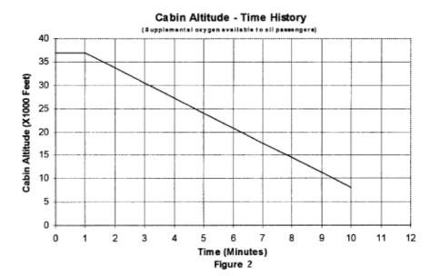
NOTE: For figure 2, time starts at the moment cabin altitude exceed 8 000 feet during depressurization. If depressurization analysis shows that the cabin altitude limit of this curve is exceeded, the following alternate limitations apply: After depressurization the maximum cabin altitude exceedence is limited 40 000 feet. The maximum time the cabin altitude may exceed 25 000 feet is 2 minutes; time starting when the cabin altitude exceeds 25 000 feet and ending when returns to 25 000 feet.
