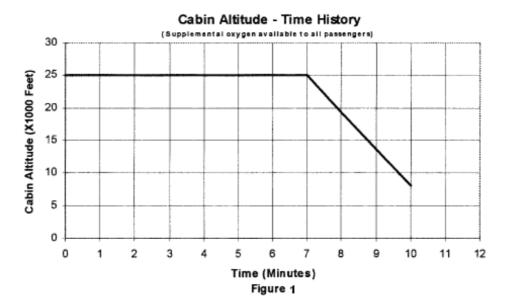
NOTE: For figure 1, time starts at the moment cabin altitude exceed 8 000 feet during depressurization. If depressurization analysis shows that the cabin altitude limit of this curve is exceeded, the following alternate limitations apply: After depressurization the maximum cabin altitude exceedence is limited 30 000 feet. The maximum time the cabin altitude may exceed 25 000 feet is 2 minutes; time starting when the cabin altitude exceeds 25 000 feet and ending when returns to 25 000 feet.
